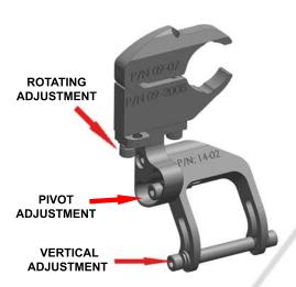
7 - Reinstall the body assembly. Be sure to include all lock washers with screws, and the lock and flat washer with the bottom socket head screw as shown above. Use the adjustments shown above to adjust the RD to your desired position. Leave enough room below bottom of mirror to allow access to top radar detector buttons. Be sure to tighten all screws after adjustments are made.
