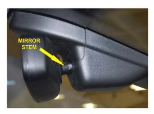
5 - While sitting in the passenger seat, place the mount over the mirror stem. Tighten the CLAMP SCREW until the mount starts to clamp onto the mirror stem. Position the mount as far forward as it will go and paralell to the bottom of the mirror before fully tightening.
